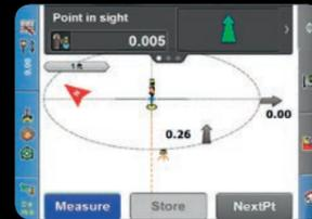
Dynamic map updates with telescope & pole positions plus bulls-eye view for fast in/out & left/right guidance
